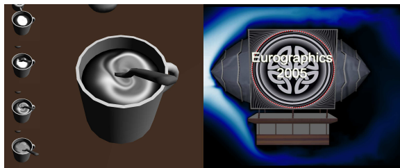
Figure 8: Images of an incompressible fluid are shown. On a 128 \times 128 grid, simulation and rendering is performed at about 450 fps on recent GPUs.
